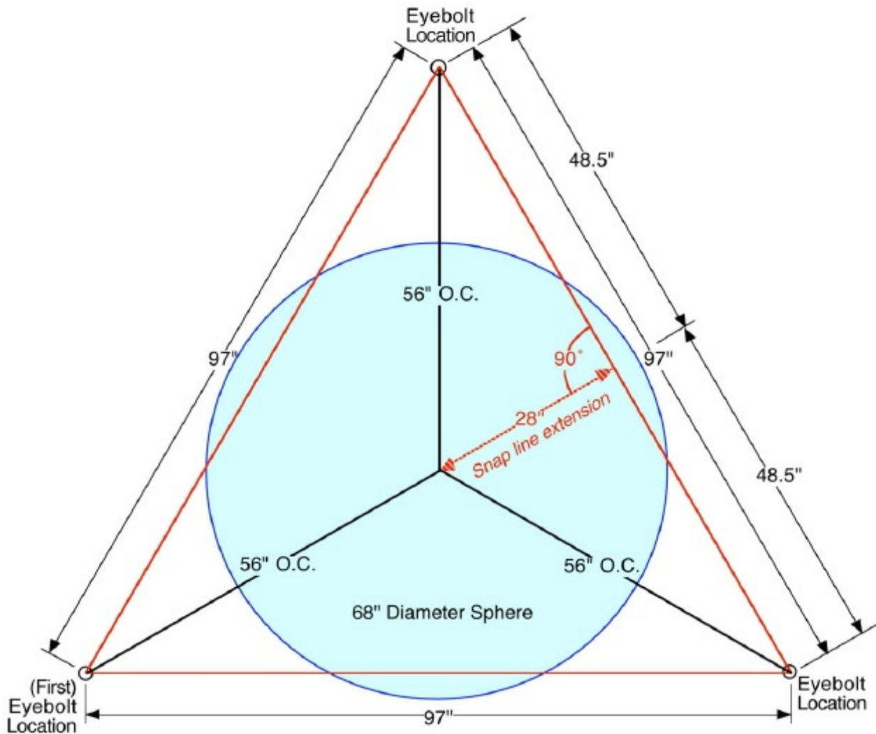
*Suspension geometry for a 68" sphere from a 20' ceiling height.*
